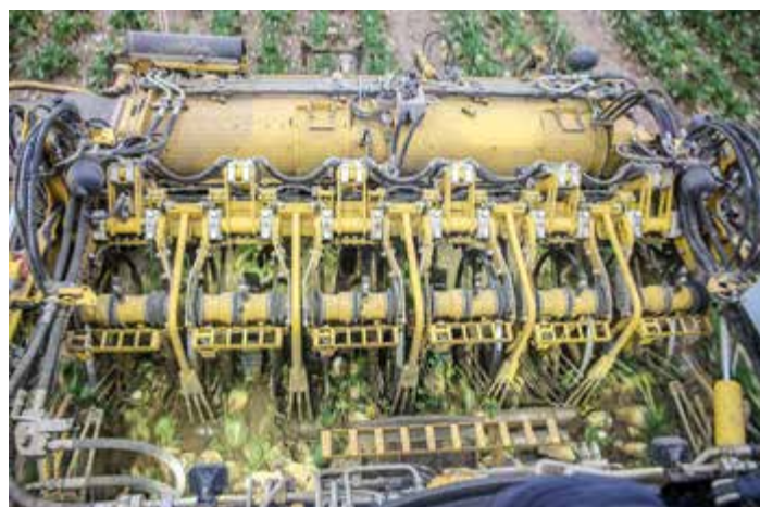
The latest RR header includes automatic individual lifter depth adjustment. The view from the cab is excellent.
